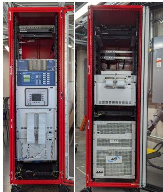
Figure 4: Typhoon HIL testbeds. Left is microgrid HIL and right is PHIL
