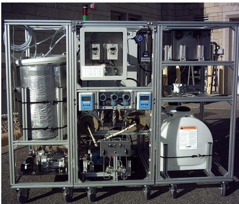
Figure 2. The portable biodiesel processing unit based on the new process
