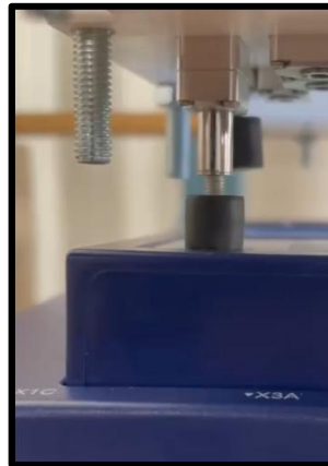
Figure 1: Actuator pressing button on controller
