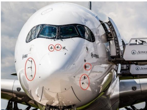
Pitot tubes and sensors on an A350
