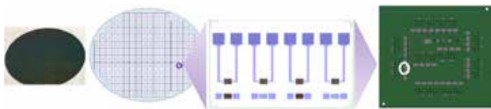
(Left to right) Wafer of sensors, sensor chip, and card with sensors
