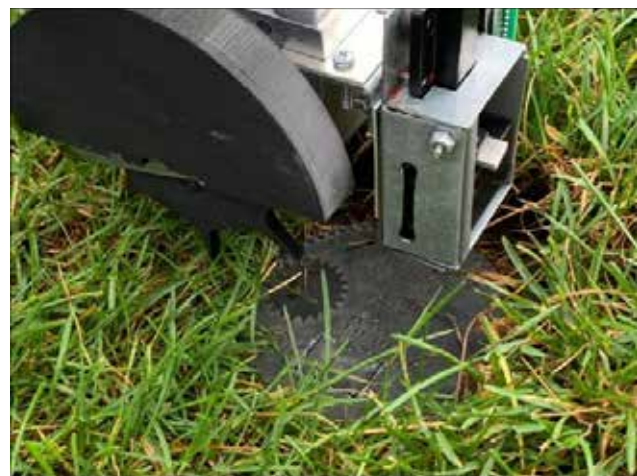
Cutting blade getting ready to trim around infrastructure
