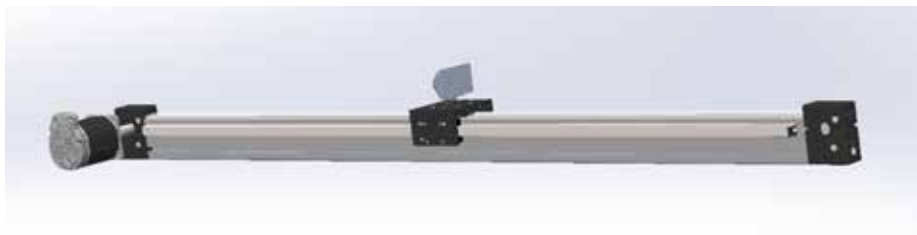
Figure 1. Shows dash cam mounted to a belt driven linear actuator and powered by an electric motor. The camera accelerates along the track and then is quickly brought to a halt to simulate 4+gs of force
